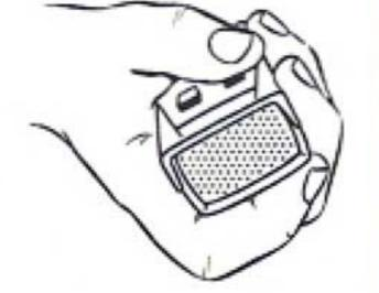
Depress "Tune" button, aim and TILT hand to LEFT to move dial pointer to left!
