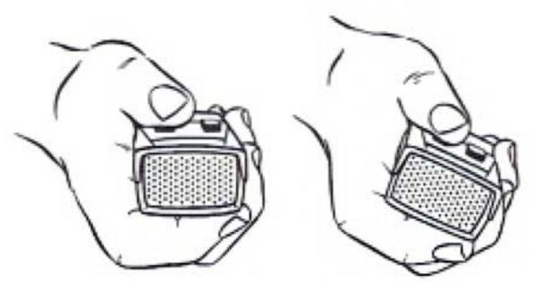
Depress "Volume" button, aim and TILT hand to left for less volume and turning set off.
