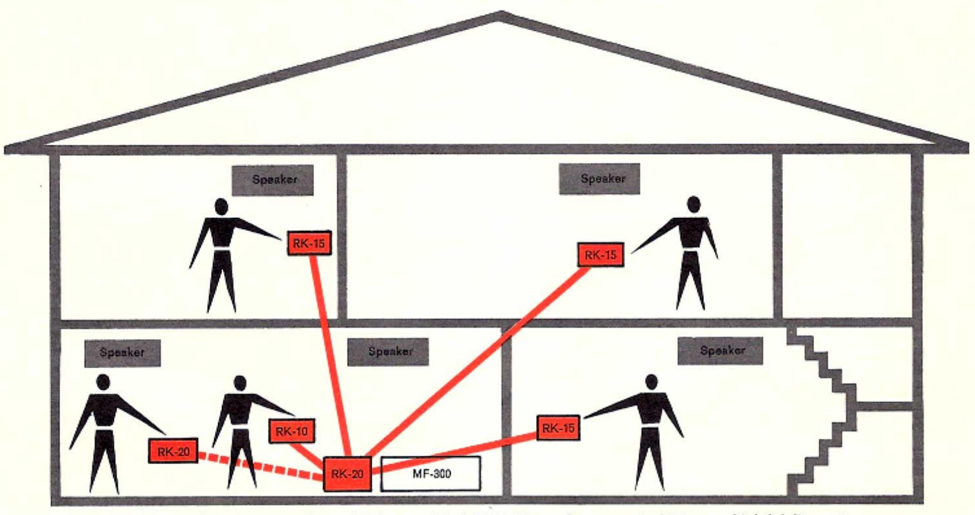
Any number of Wire Remote Control Adaptors (Model RK-15) can be connected into your high fidelity system.
